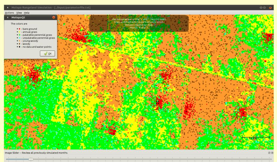
**Screen-shot (Fig. C)** of a simulation run on real satellite data. Each pixel represents a dominating vegetation type. Fence-line effects are visible due to different paddocks. Clusters of bare ground (red) appearing around watering points are a combined result of grazing and trampling. The large diagonal line is an artifact from a road crossing the area.
